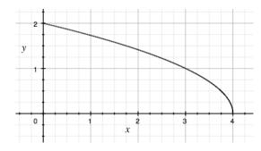
Note that D is bounded on the left by x=0, and the rightmost point in R is at (x,y)=(4,0). The parabola  $x=4-y^2$  is also described by the equation  $y=\sqrt{4-x}$ ; just solve the equation for y in terms of x. So for a given value of x between 0 and 4, y can vary from 0 to  $\sqrt{4-x}$ . We now have the limits of integration.
